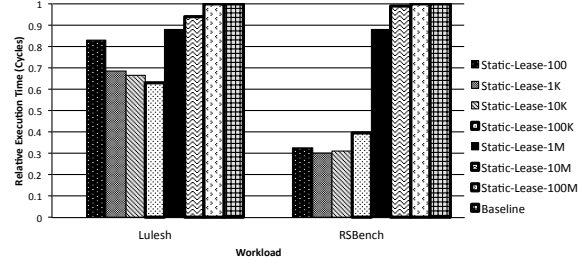
Figure 5. Impact of the lease length on execution time, normalized to the baseline (no self-invalidating TLB).
